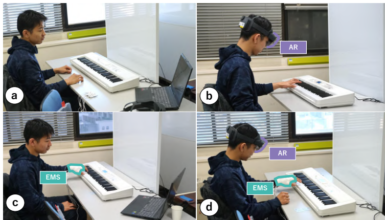
Fig. 8. Participant setup during the experiment for each condition. (a) Video condition: learning by watching a video of the instructor's hand. (b) AR condition: learning by following an AR hand model. (c) EMS condition: learning with EMS feedback while watching the video. (d) AR \times EMS condition: learning with both AR hand model and EMS feedback.
