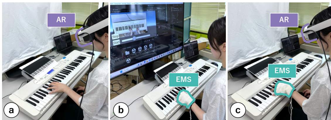
Fig. 11. Participants in each condition. (a) AR condition: learning by following an AR hand model. (b) EMS condition: learning with EMS feedback while watching a video. (c) AR \times EMS condition: learning with both AR hand model and EMS feedback.
